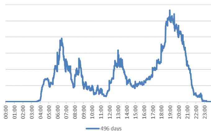
Figure ES-3: Average load profile for all complete days of data recorded during this study.
