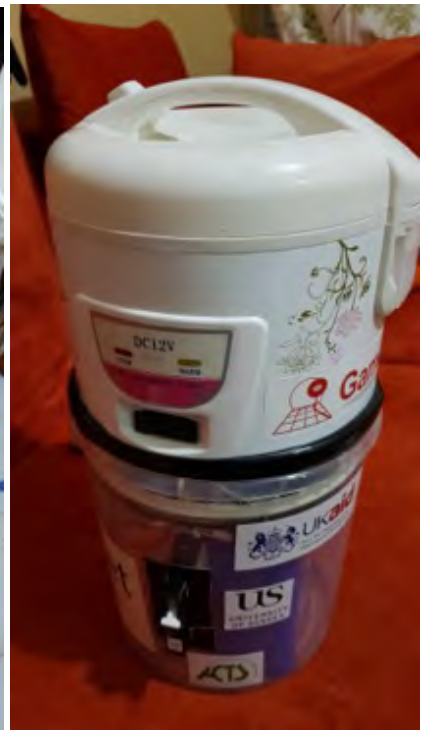
Figure 14: The 'bucketization' of the eCookBucket. A simple household bucket was used to extend the body of the DC rice cooker around the battery. The only other component is a DC circuit breaker, which also functioned as an on/off switch.
