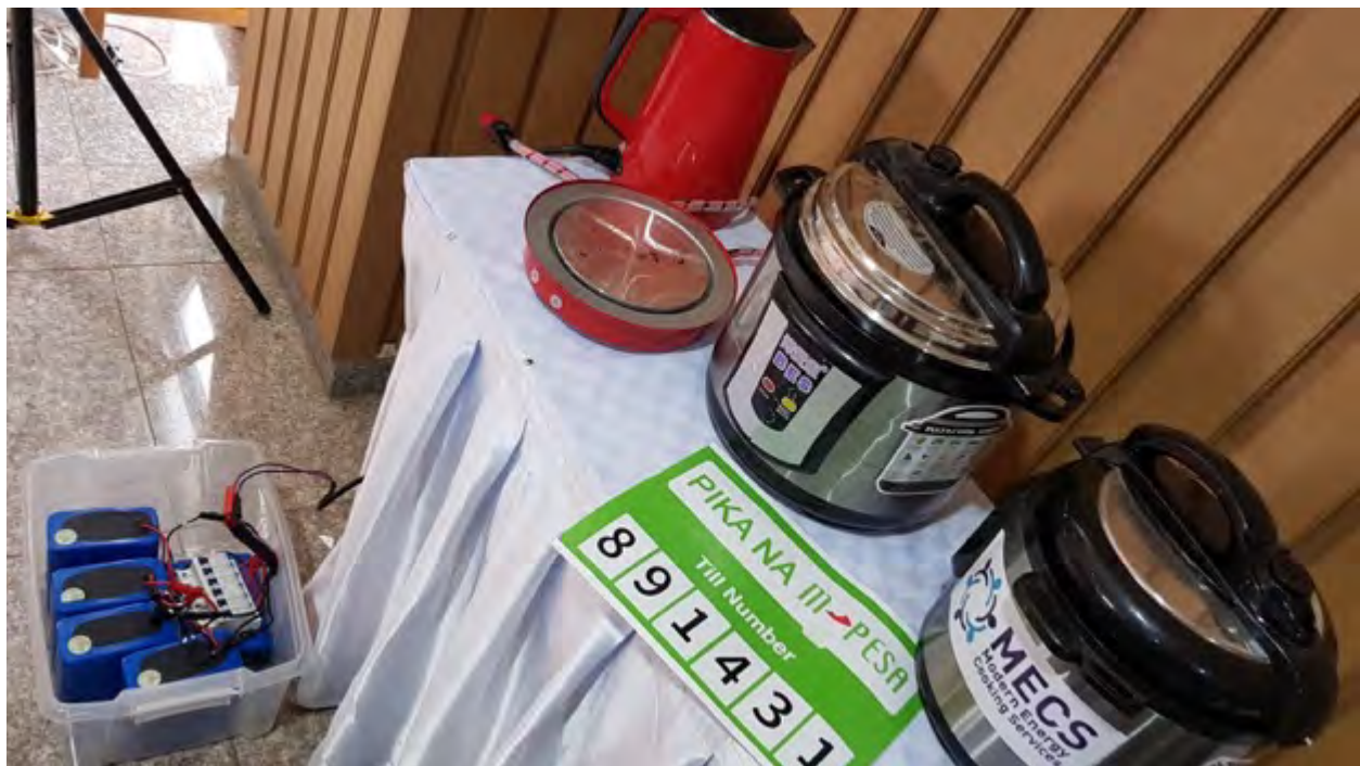
Figure 20: A range of DC cooking appliances manufactured by Tesga Power on display at the MECS East Africa Launch in May 2019 in Nairobi Kenya. From top to bottom: a DC kettle, DC hotplate, 5 litre DC EPC and 2.8 litre DC EPC. On the left is the 1.2kWh LiFePO4 battery bank from the eCookBox.
