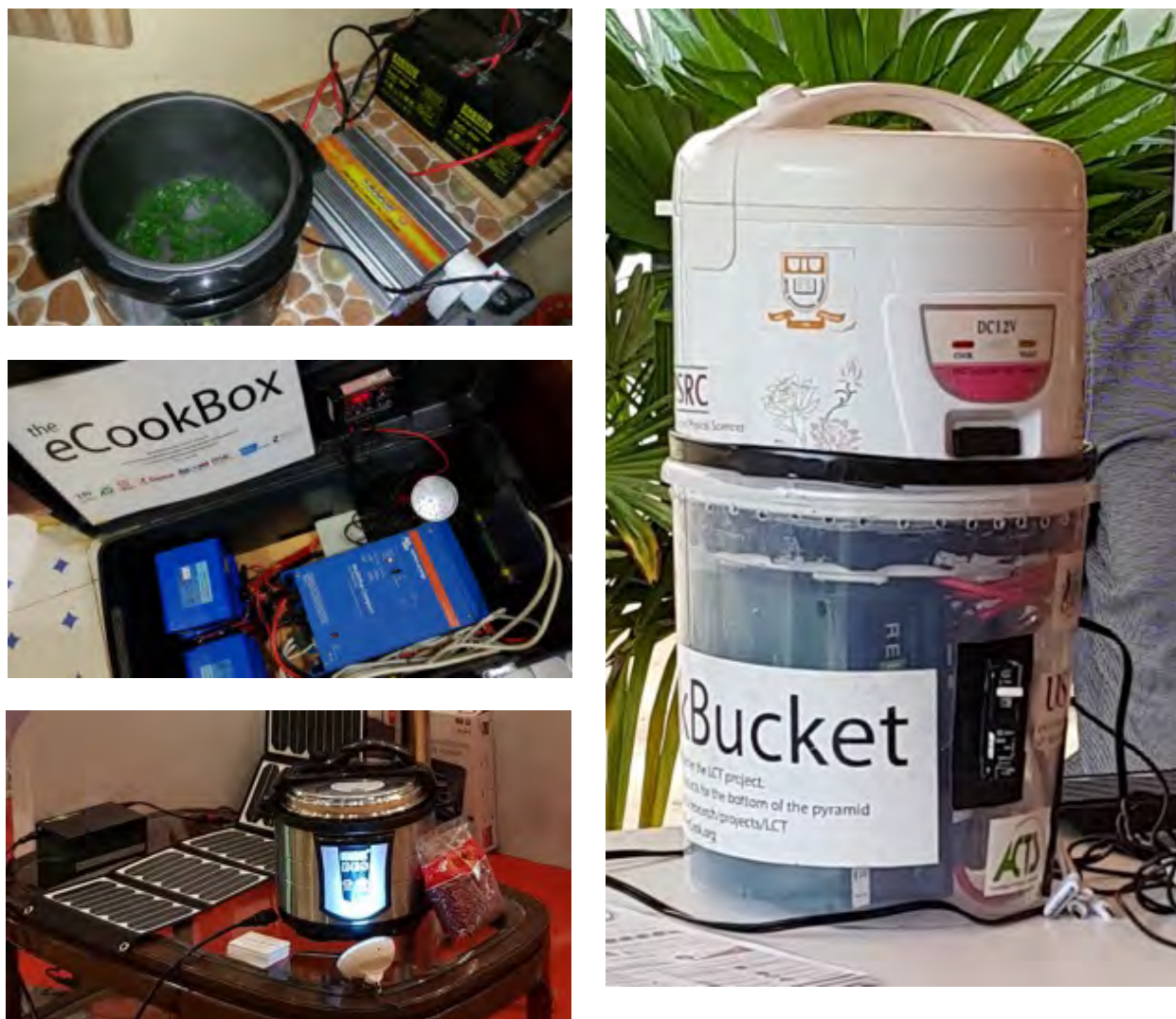
Figure ES-1: The evolution of the eCook Kenya Prototypes: the lead acid AC Mark 1 (top left), the LiFePO4 AC Mark 2 eCookBox (middle left), the DC battery-integrated LiFePO4 Mark 3 eCookBucket (right) and the ultra-efficient DC LiFePO4 Mark 4 (bottom left).
