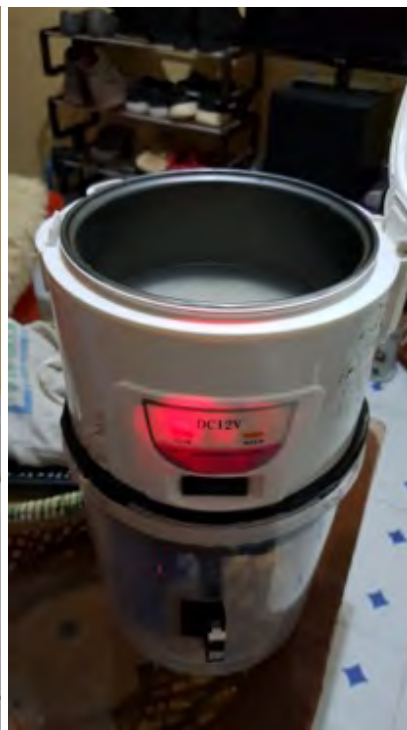
Figure 14: The 'bucketization' of the eCookBucket. A simple household bucket was used to extend the body of the DC rice cooker around the battery. The only other component is a DC circuit breaker, which also functioned as an on/off switch.
