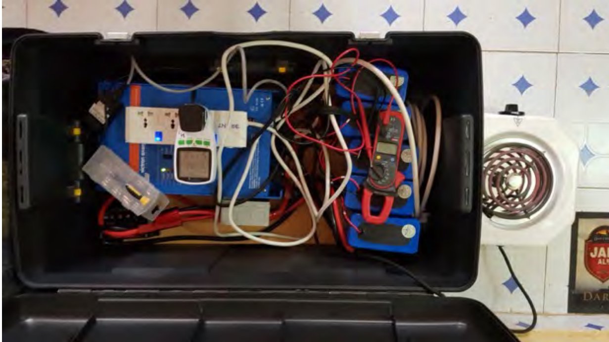
Figure 6: Testing the eCook Kenya Mark 2 Prototype with an AC electric hotplate.
