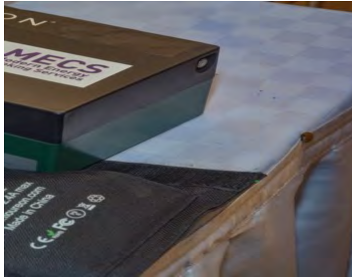
Figure 19: The modified golf-cart battery after removing the battery terminals and rebranding.
