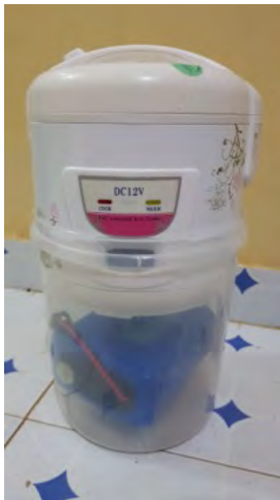
Figure 14: The 'bucketization' of the eCookBucket. A simple household bucket was used to extend the body of the DC rice cooker around the battery. The only other component is a DC circuit breaker, which also functioned as an on/off switch.
