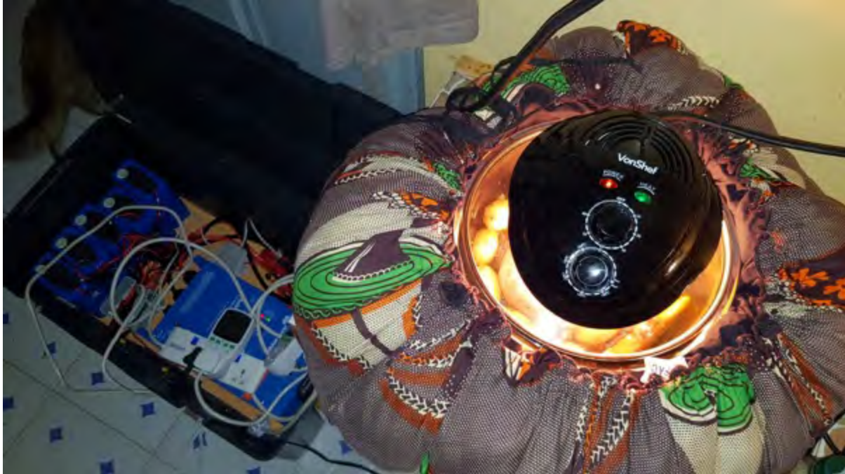
Figure 10: Experimenting with adding insulation to a halogen oven to reduce energy losses to enable more cooking to be done on the battery-supported system.
