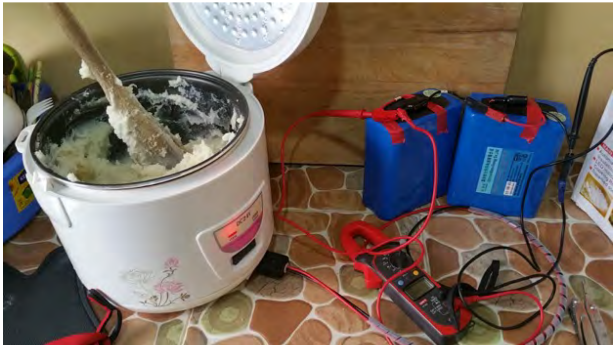
Figure 13: Experimenting with cooking ugali with the DC rice cooker. The non-stick pot was very easy to clean, but the temperature sensor designed to turn the appliance onto warm mode after rice had cooked could not be overridden without taking the appliance apart, meaning that cooking times were extended considerably.
