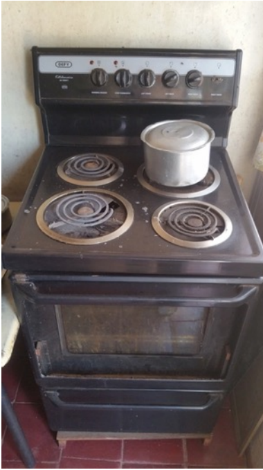
Figure 9: The four-plate stove – the aspirational cooking device for many. Capable of heating four pots, baking and grilling simultaneously. They are typically fitted with 40-60 amp circuit breakers, as they can consume up to 10kW.
