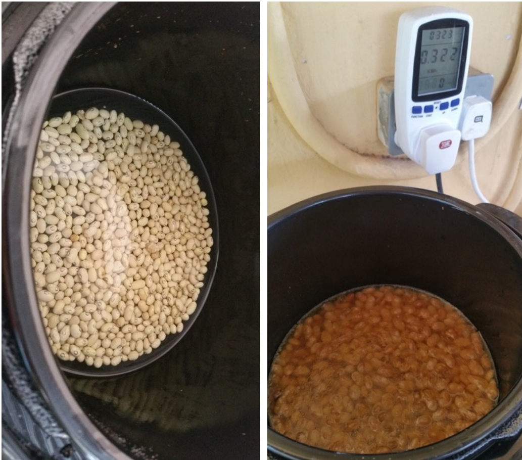
Figure 30: The EPC can reduce the time for cooking beans by up to half and the energy by up to 80%. However, correctly judging the amount of water and the cooking time is challenging, even for people who have cooked beans many times, as you cannot see (or smell) inside without depressurising. These beans consumed a total of 0.381kWh:
