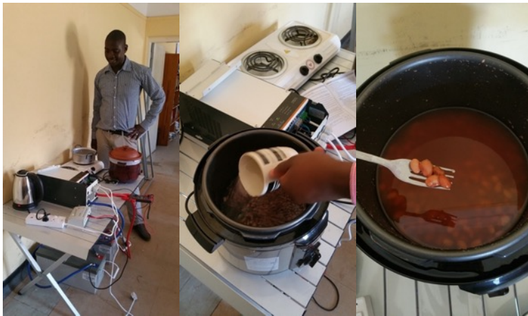
Figure 44: Testing the eCook Zambia prototype by cooking beans on the E.P.C. at the CEEEZ office. The oversized battery bank and high-quality pure sinewave inverter were more than capable of handling the relatively small loads from the portable electric cooking appliances.
