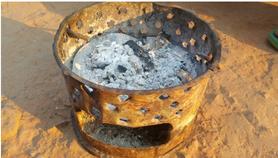
Figure 4: the mbaula – Zambia’s most popular charcoal stove. It’s very cheap to make, portable and so widely available that many people are unaware that other charcoal burning stoves even exist. Today, it can be found in most urban Zambian homes, either as the main cooking device or at least as the backup for when the power goes out. However, its thin walls allow heat to escape all around. Small pots simply sit on top of the charcoal, allowing more heat to escape up the sides of the pot, meaning that very little actually makes it into the food.
