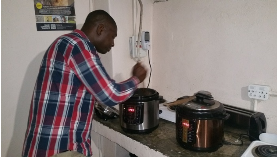
Figure 31: The beans and impala were cooked together in two separate EPCs. They were accompanied by nshima cooked on the hotplate/kettle (see Figure 14 for recipe). The sauce for the beans was also prepared on the hotplate, then blended in with the beans on the EPC. The meal served 6 people and the total energy consumption was 1.474kWh:
