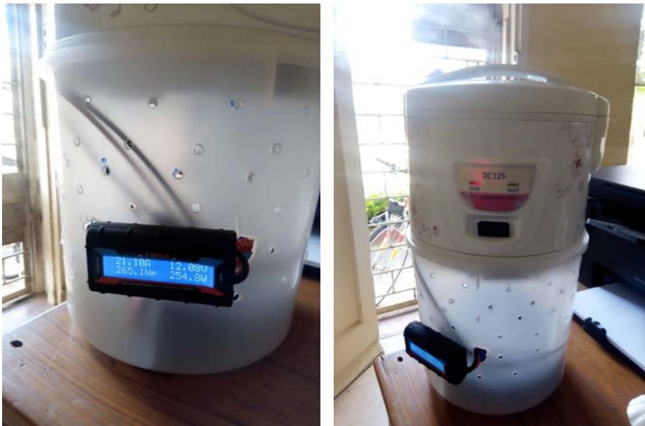
Figure 60: The simple eCookBucket was merely an actual bucket paired with a DC rice cooker obtained as a sample from a Chinese factory. Together, they created a very crude DC battery-integrated cooking appliance.
