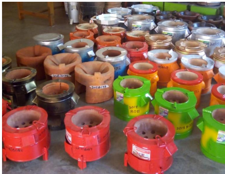
Figure 3 Locally made improved stoves in Uganda
