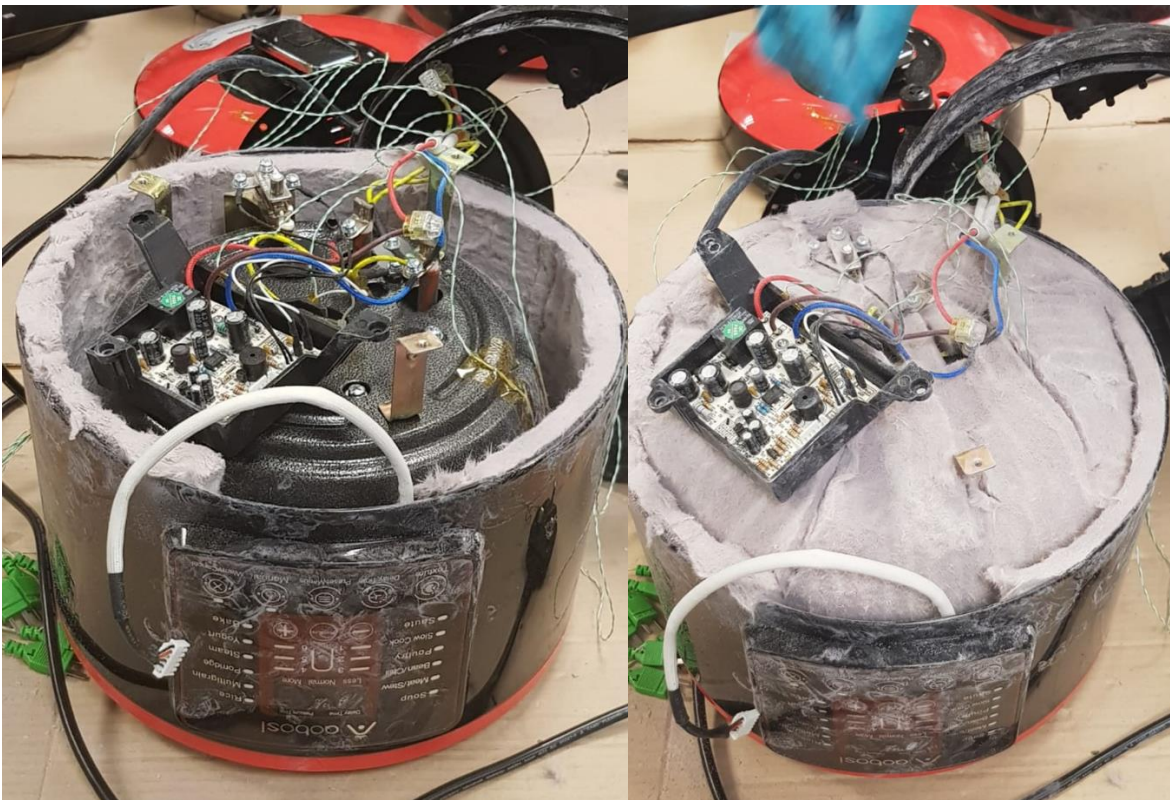
Figure 2 During installation. Handling Pyrogel XTE insulation required full PPE - photographs of view from beneath the EPC with base support and cover removed. Other Aspen Aerogels products have different handling qualities.
