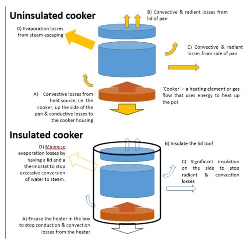
Figure 3: Heat loss mechanisms mitigated by insulating the cooking pot and heating device. Adapted from Batchelor et al. [25].
