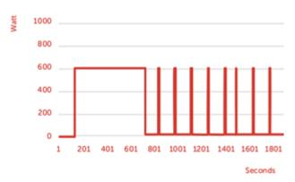
Figure 4: Typical load profile for a 700W rated EPC on a half hour cooking cycle [26].
