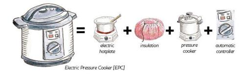
Figure 5: The fundamental components of an EPC.
