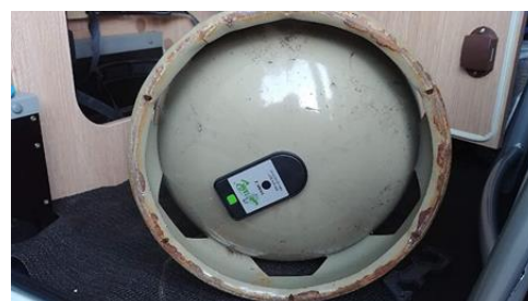
Figure 1: MOPEKA's ultrasonic sensor
