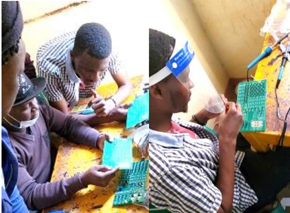
Figure 14: Assembly of an early version prototype of the LTO BMS circuit.
