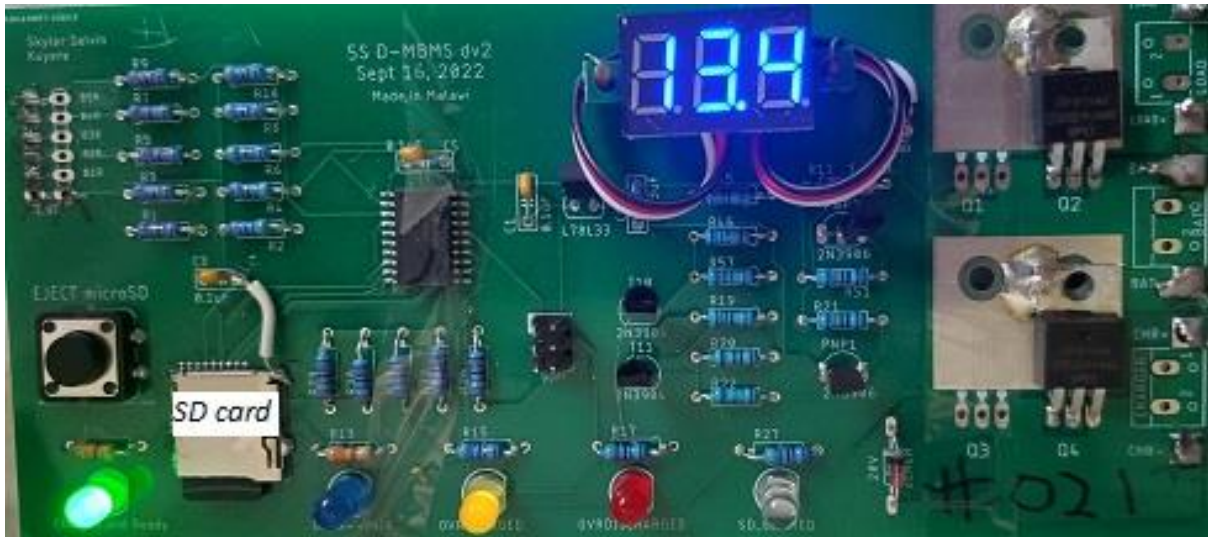
Figure 15: End-of-project version of prototype of the LTO BMS circuit with data collection capabilities.
