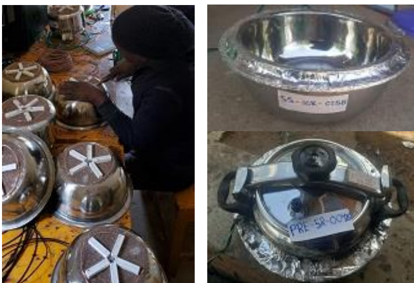
Figure 3: Cookers with resistive heating elements being locally assembled in Malawi. Both simple cooker and pressure cookers were assembled and distributed.
