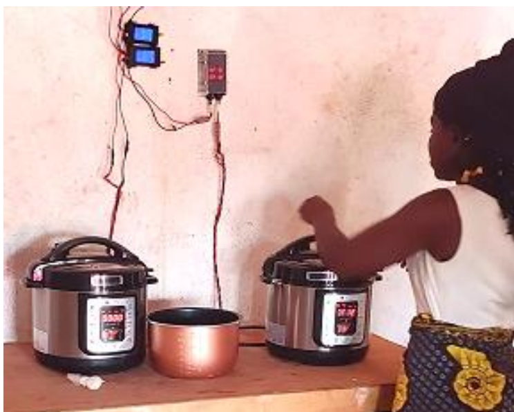
Figure 13: Incentivized demonstration of solar electric cooking at the M'bangombe women's solar shop. The small meters with the blue screens record instantaneous voltage, current and power and record cumulative energy use
