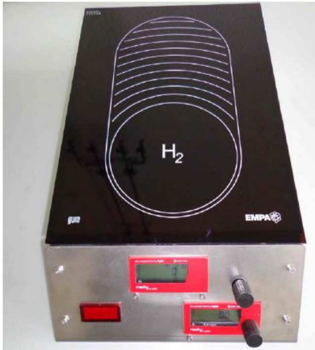
Figure 2: Assembled catalytic hydrogen combustion cooker (Source: Mukelabai et al., 2022, p. 9)
