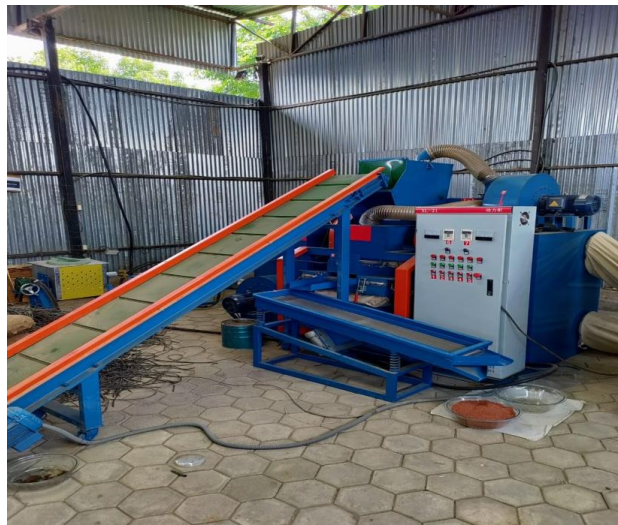
Figure 47 Cable granulator machine used for copper and aluminum extraction
