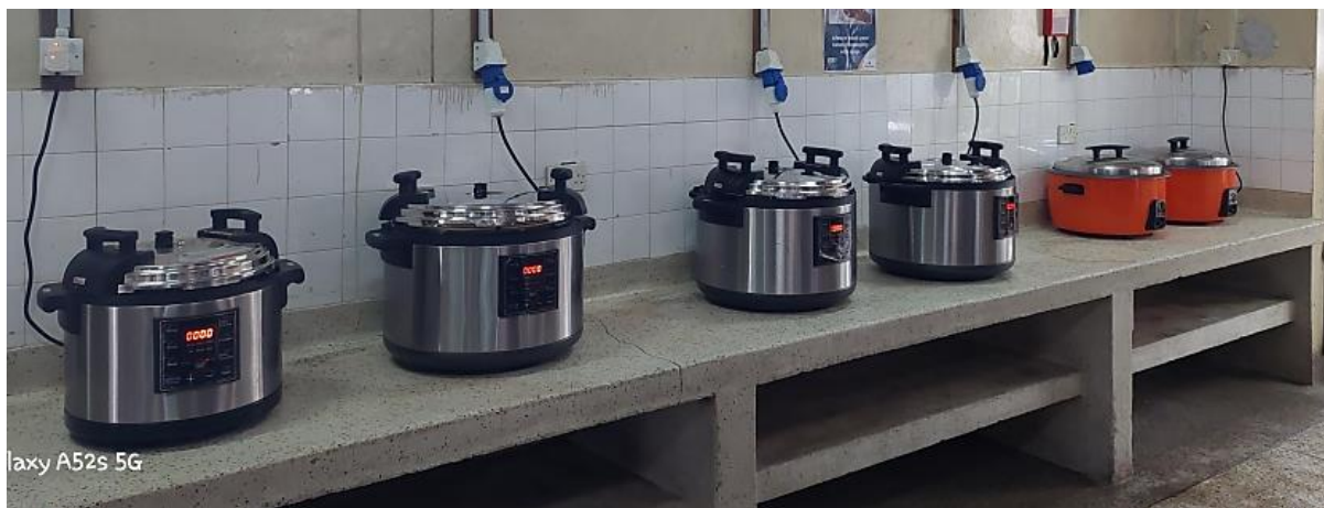
Figure 1: From left - 25-liter EPC, three 40-liter EPCs, and two 16-liter rice cookers.
