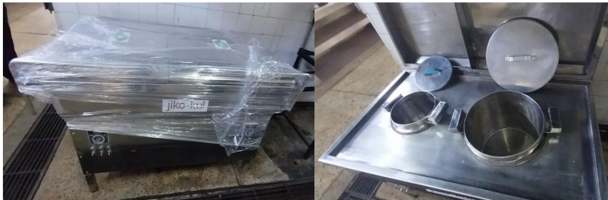
Figure 5: 58-Liter 2-in-1 Multipurpose Electric Cooker (Jiko Kul) at IESR's Kitchen.
