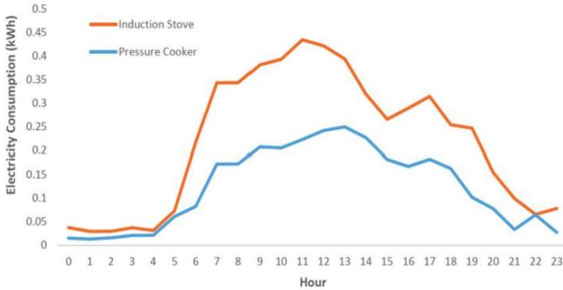
Figure 4.5: Average hourly load profiles for EPCs and induction cookers from a previous study. Developer 2, 2023 [2].
