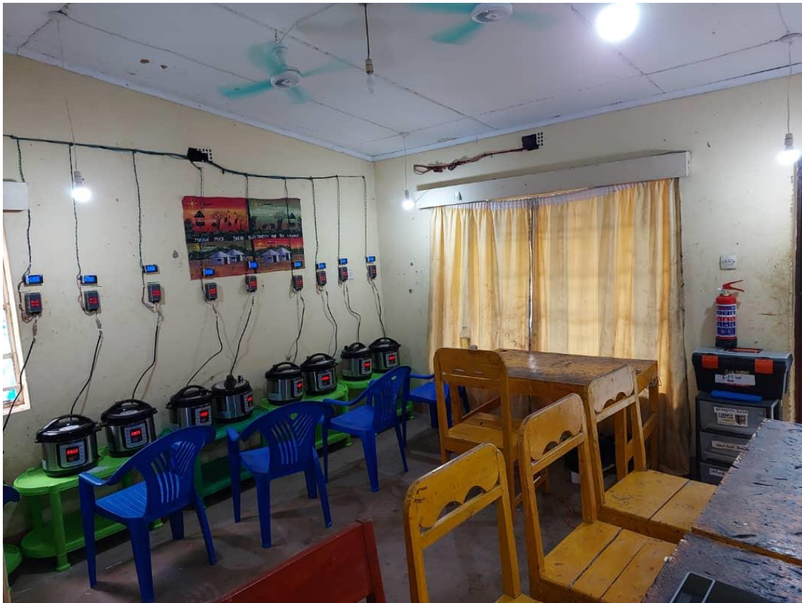
Figure 2: Testing set-up for evaluating the cooking performance of the initial design of an off-grid DDS solar electric cooking system with a DC-EPC.
