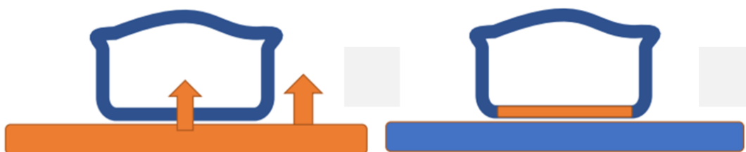
Figure 11: Hot resistive element passing heat to the pot and escaping up the sides of the pot (left); induction generates heat in the bottom of the pot only (right) (Credit: Dr Simon Batchelor).
