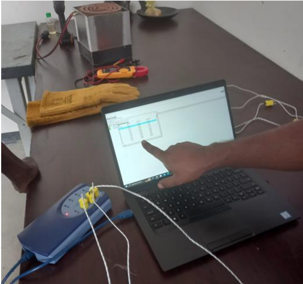
Figure 5: Omega Engineering Limited 8 CH T/C USB DATA ACQ MODULE
