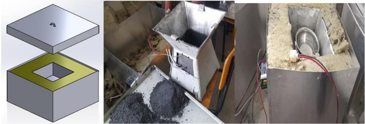
Figure 19: Alternative cooking stove design to stop upper heat loss
