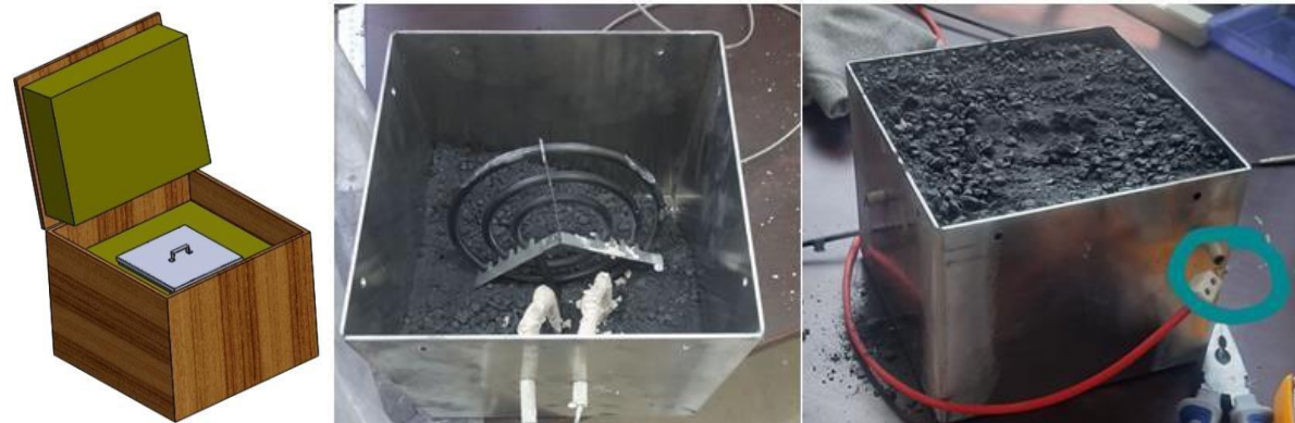
Figure 16: only magnetite without internal aluminum cells
