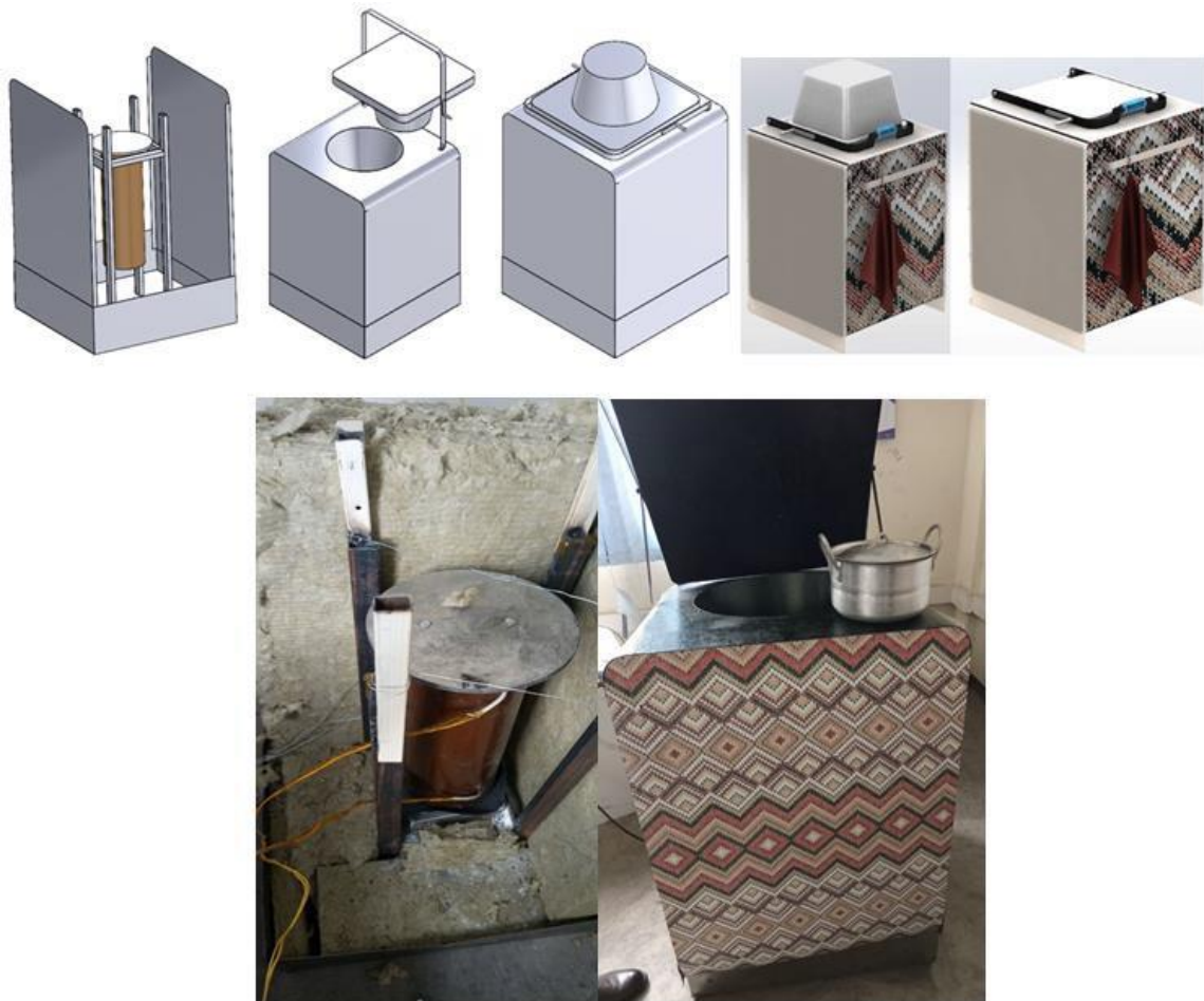
Figure 26: New design to solve the upper insulation during and after cooking
