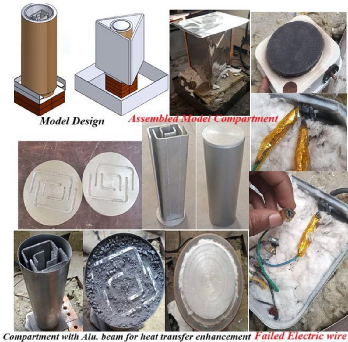
Figure 31: Improved Aluminum heat transfer structure and vacuum panel use. Failed electric plate
