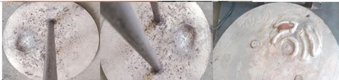
Figure 30: Aluminum disks and rods, melted aluminum at bottom near heating
