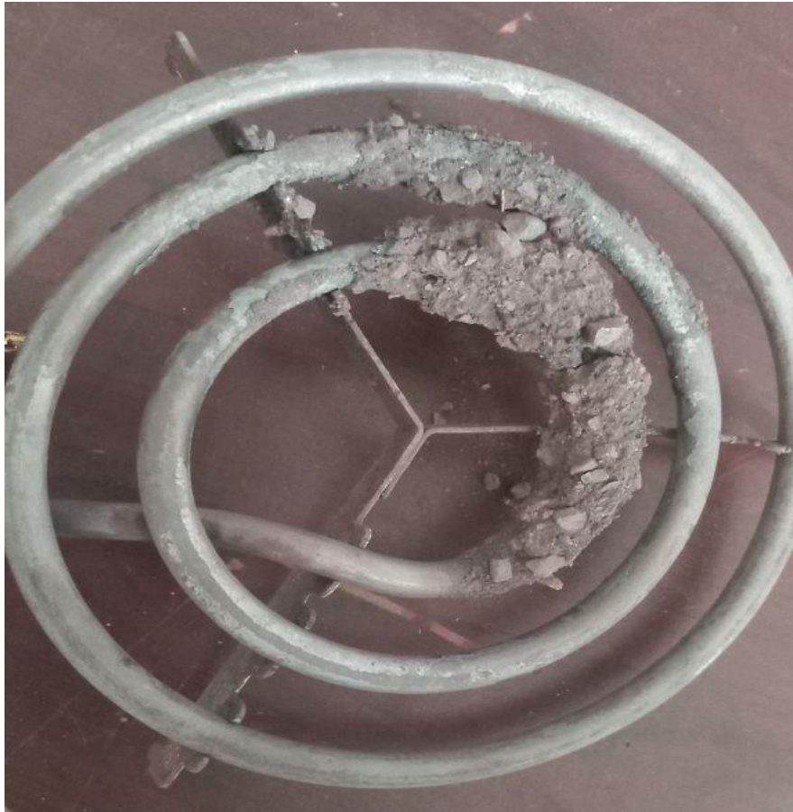
Figure 18: Heat coil failure and aggregation
