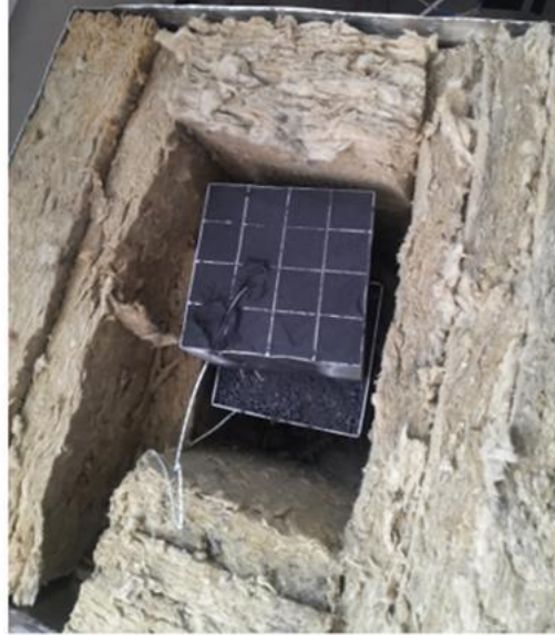
Figure 20: New version with upper insulated lid to contain heat loss
