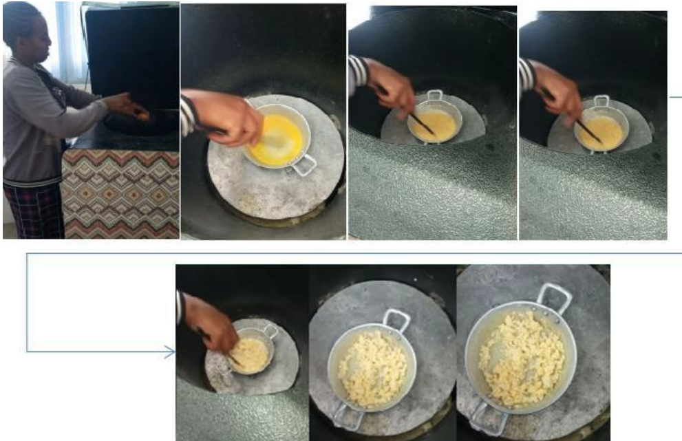
Figure 29: Scrambling egg using stored heat by magnetite
