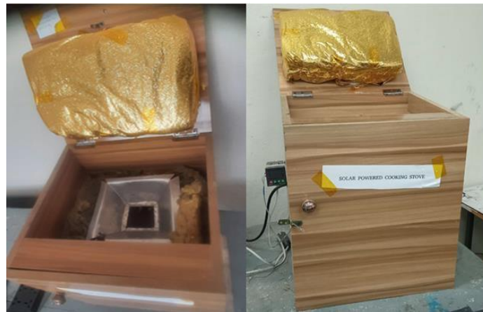
Figure 17: alternative design with 20 cm Rockwool
