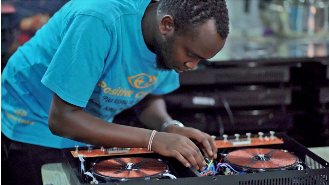
The image above shows one of the Verst Carbon staff members embedding the IoT and PAYGO card into a Positive Cooker double-burner induction cooker
