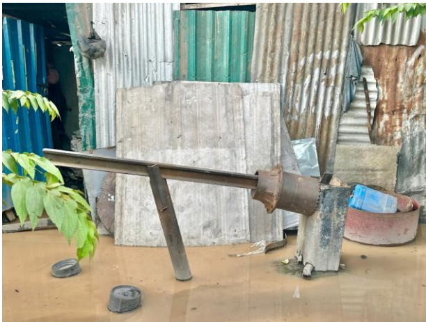
Improvised tool which can be used for bending/ rolling
